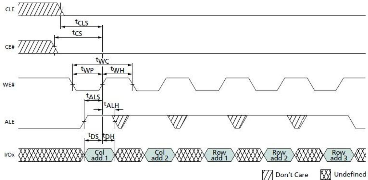
**Asynchronous Data Input**
