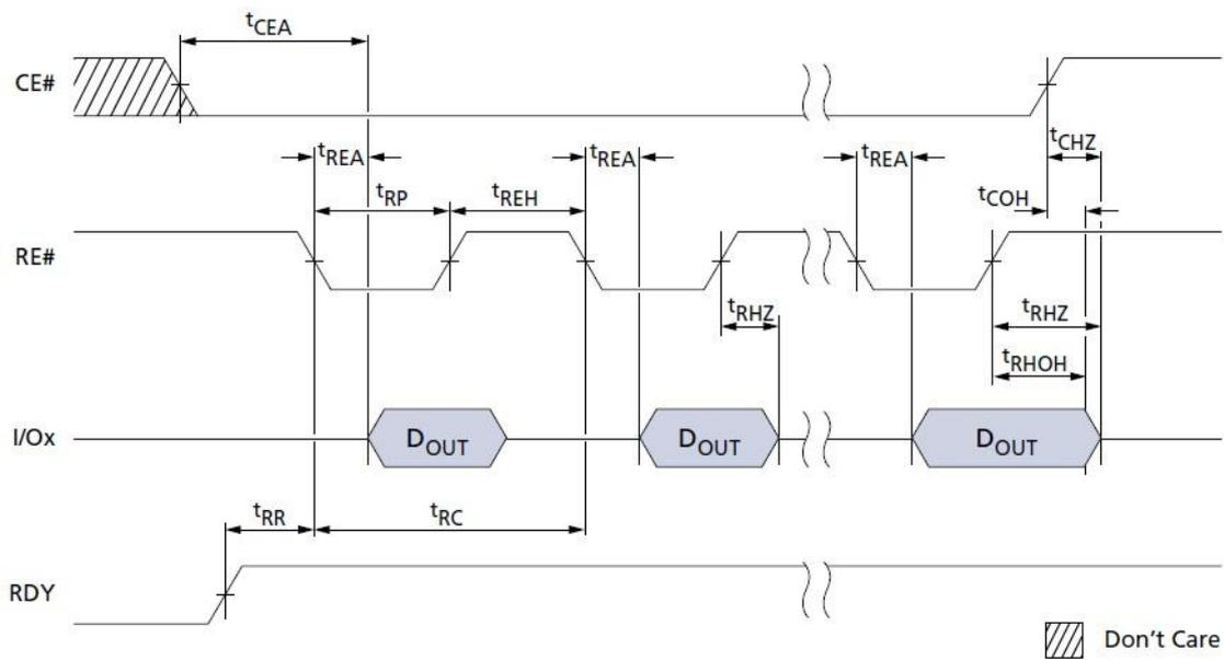
**Asynchronous Data Output Cycles (EDO Mode)**
