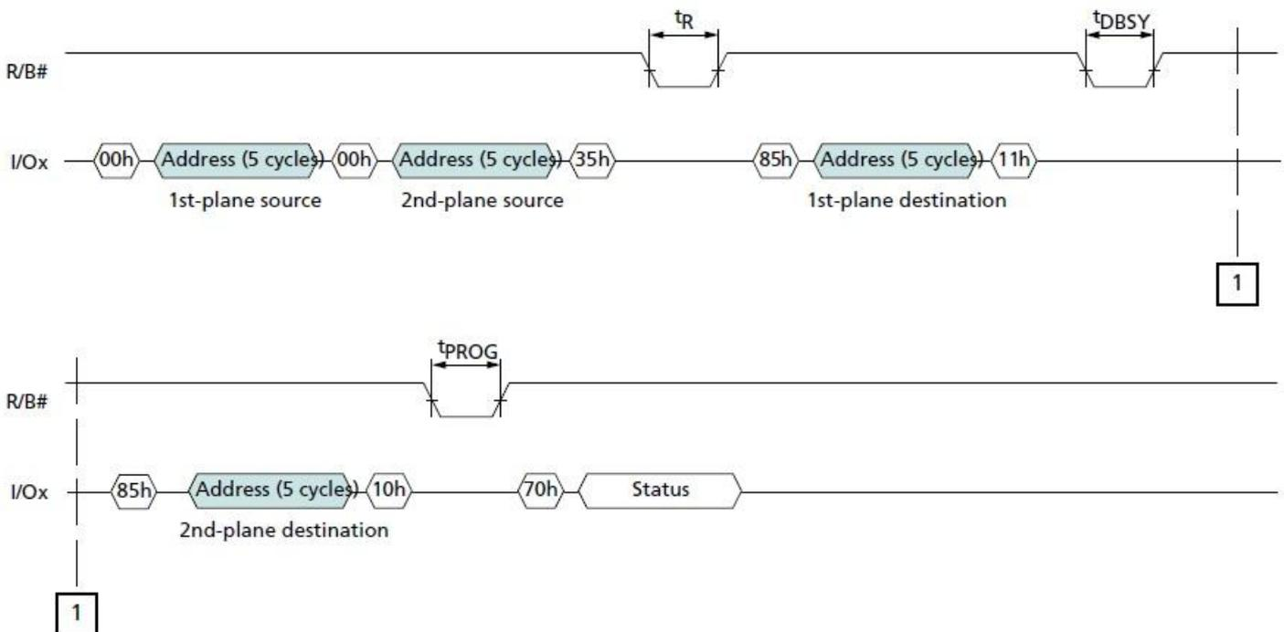
**TWO-PLANE INTERNAL DATA MOVE with TWO-PLANE RANDOM DATA READ**
