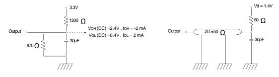
(Fig. 1) DC Output Load Circuit
