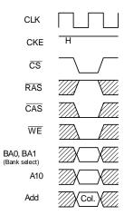
Fig. 4 Column address and write command
