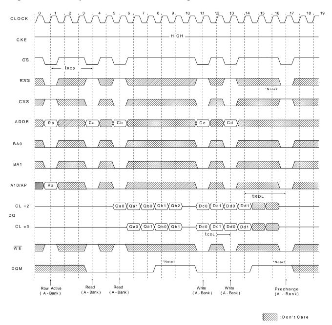
Note: 1. To Write data before burst read ends. DQM should be asserted three cycles prior to write command to avoid bus contention.
