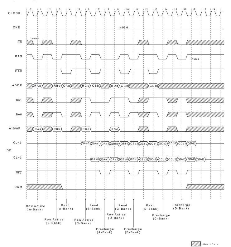
Note: 1.  $\overline{\text{CS}}$  can be don't cared when  $\overline{\text{RAS}}$ ,  $\overline{\text{CAS}}$  and  $\overline{\text{WE}}$  are high at the clock high going edge.
