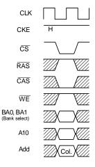
Fig. 5 Column address and read command
