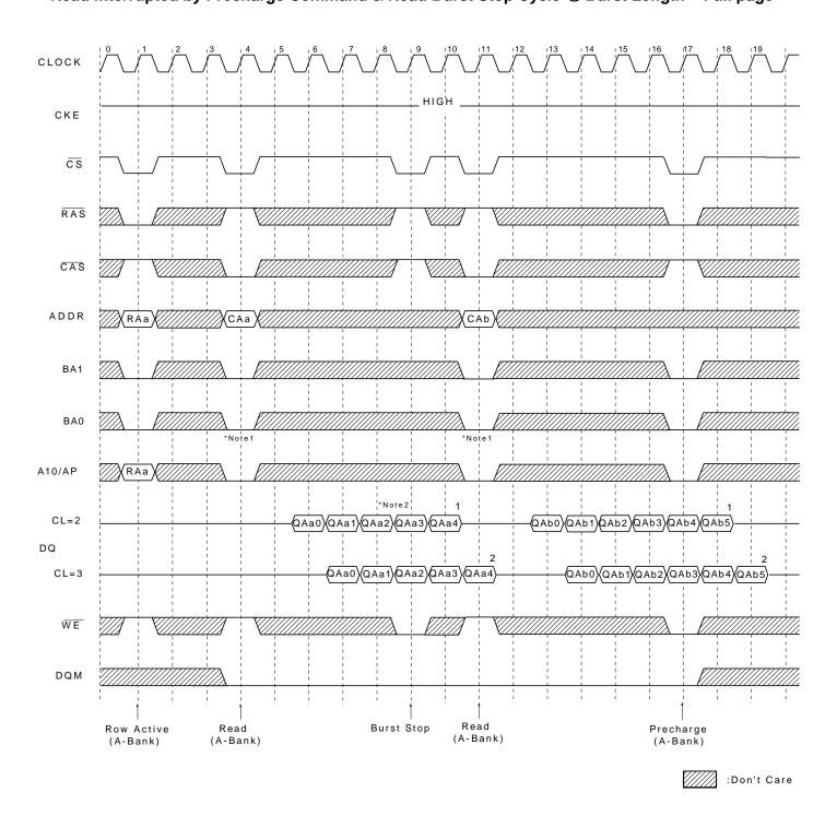
1. About the valid DQs after burst stop, it is same as the case of  $\overline{RAS}$  interrupt. Both cases are illustrated above timing diagram. See the label 1, 2 on them. But at burst write, Burst stop and RAS interrupt should be compared carefully. Refer the timing diagram of "Full page write burst stop cycles".
