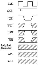
Fig. 8 Burst stop command
