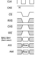
Fig. 2 Row address stroble and bank active command
